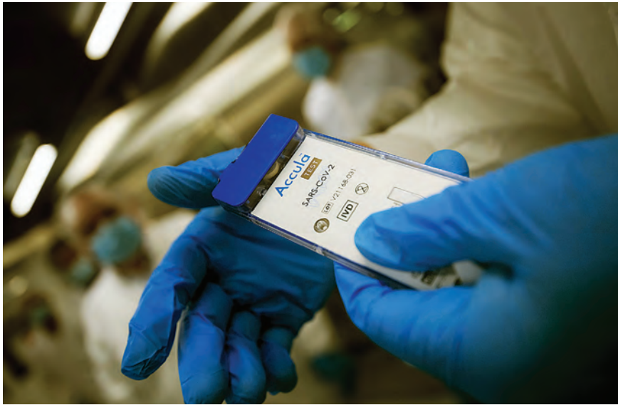
Thermo Fisher's reusable Accula Dock streamlines RT-PCR testing using a fully integrated, single-use microfluidic test cassette
